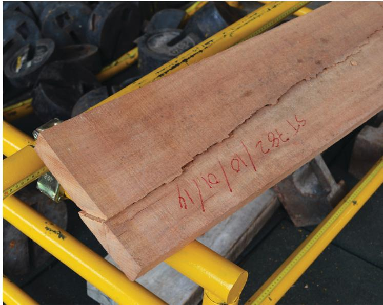
Figure 12 Horizontal split failure of a scaffold board
