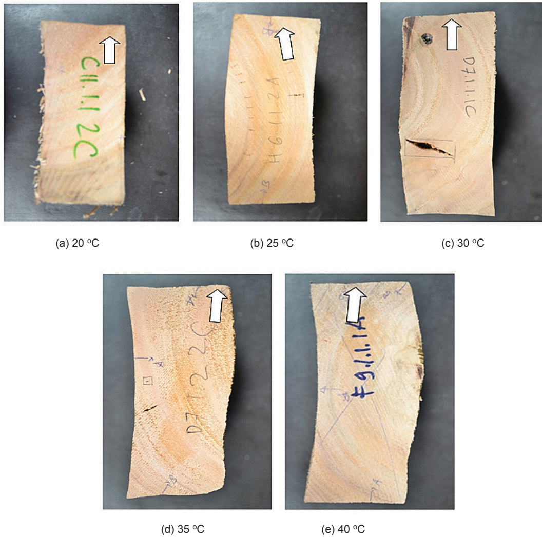
Figure 7 Washboarding on radial surface (marked with white arrow) of the board dried at different temperatures
