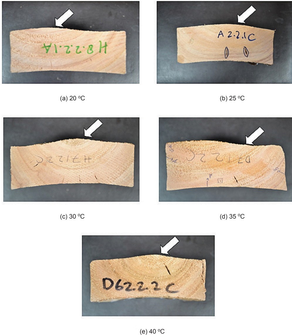
Figure 6 Corrugation on tangential surface (marked with white arrow) of the boards dried at different temperatures
