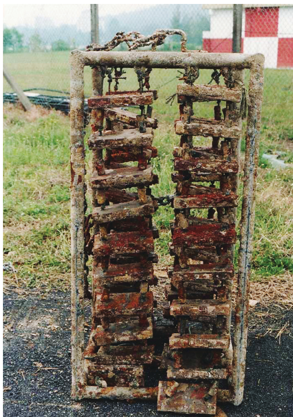
Figure 1 Test blocks specimens after 6 months exposure at Lumut, Perak
