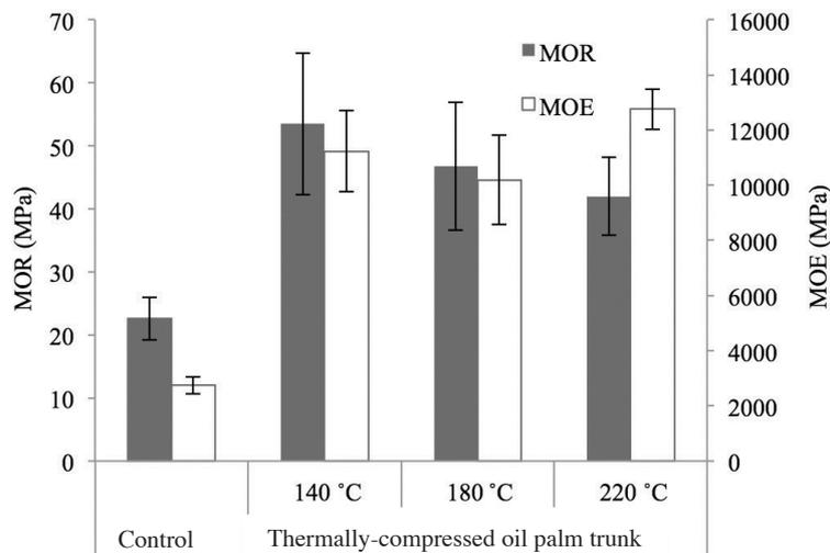
**Figure 1** Modulus of rupture (MOR) and modulus of elasticity (MOE) of control and hot-pressed oil palm wood
