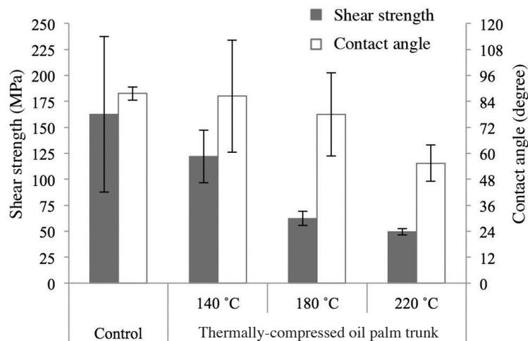
**Figure 7** Shear tested bond strength and contact angle of control and hot-pressed oil palm wood
