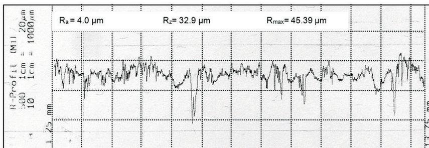
**Figure 5** Representative surface roughness profiles at different hot press temperatures;  $R_a$  = average roughness,  $R_z$  = peak-to-valley height,  $R_{max}$  = maximum roughness
