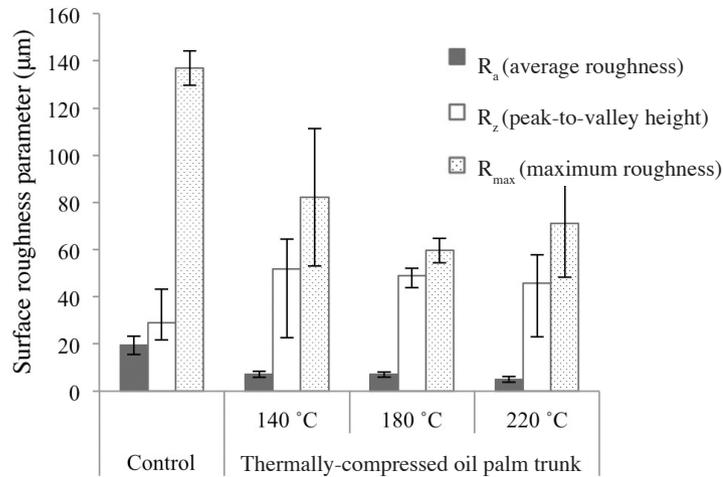
**Figure 6** Surface roughness of control and hot-pressed oil palm wood
