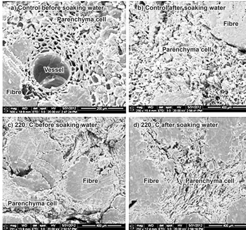
**Figure 4** Micrographs of cross-sections of control and hot-pressed samples (220 °C), before and after water soaking
