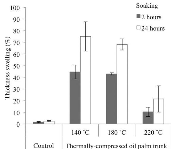
**Figure 3** Thickness swelling of control and hot-pressed oil palm wood soaked for 2 and 24 hours
