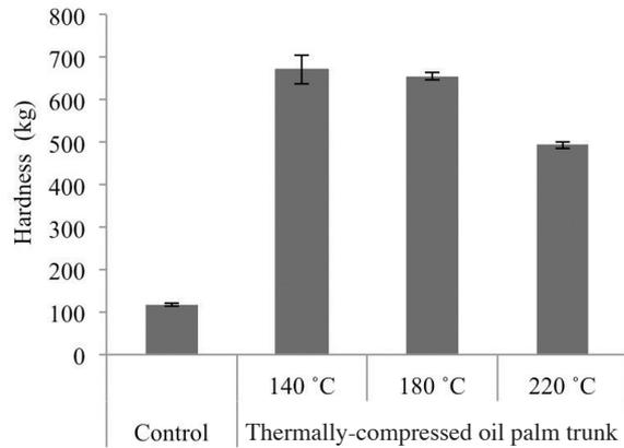
**Figure 2** Hardness of control and hot-pressed oil palm wood
