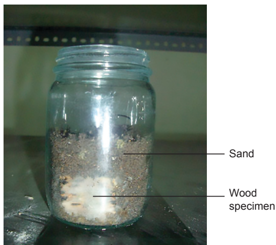
Figure 1 Container used in the subterranean termite test
