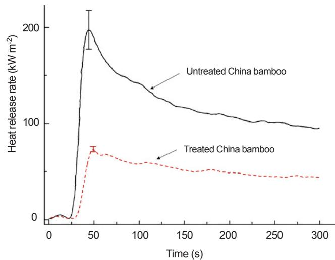
Figure 7 Heat release profiles of untreated and treated China moso bamboo
