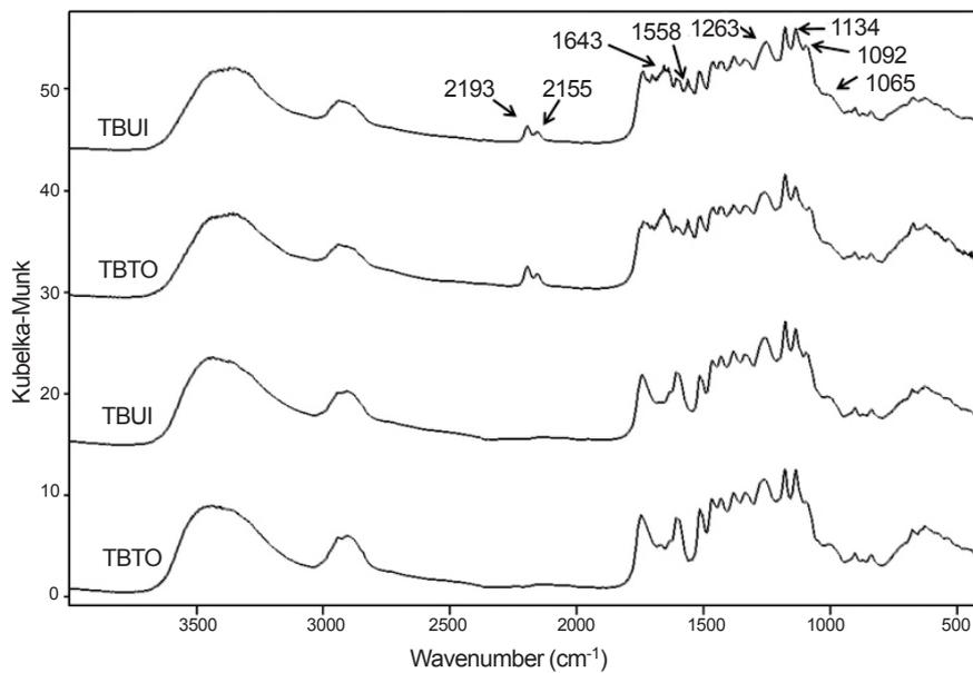
**Figure 2** FTIR spectra of Dricon-treated Taiwan moso bamboo, TBUI = outside of untreated specimen, TBUI = inside of untreated specimen, TBTO = outside of treated specimen and TBUI = inside of treated specimen)
