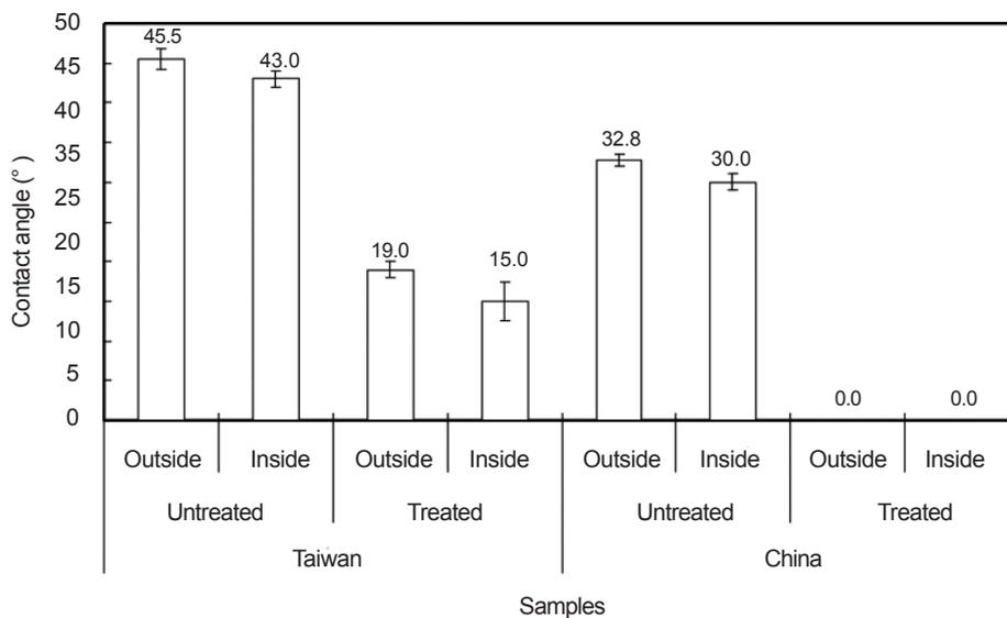
**Figure 5** Changes in contact angle on surface of Dricon-treated moso bamboo
