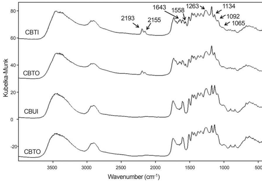
**Figure 1** FTIR spectra of Dricon-treated China moso bamboo (CBUI = outside of untreated specimen, CBUI = inside of untreated specimen, CBTO = outside of treated specimen and CBTI = inside of treated specimen)
