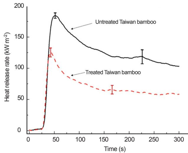
Figure 6 Heat release profiles of untreated and treated Taiwan moso bamboo
