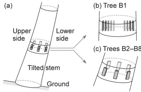
**Figure 4** Measurement of released strain of surface growth stress and specimen preparation, (a) measuring points of released strain, (b) specimen preparation for radial distribution of tensile Young’s modulus, (c) specimen preparation for peripheral distribution of material properties
