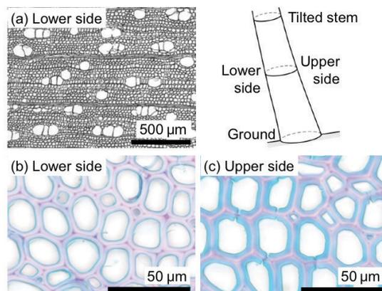
**Figure 5** Observation of *Styrax tonkinensis* wood by optical microscopy, (a) and (b) fibres in the lower side of a tilted stem, (c) fibres in the upper side
