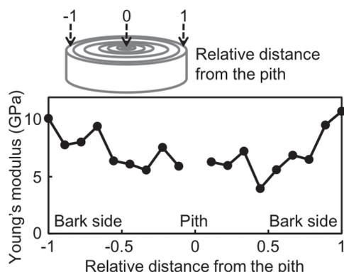
**Figure 8** Radial distribution of tensile Young's modulus. X axis shows the relative positions from pith to bark, 0 = position of the pith, 1/-1 = outermost side
