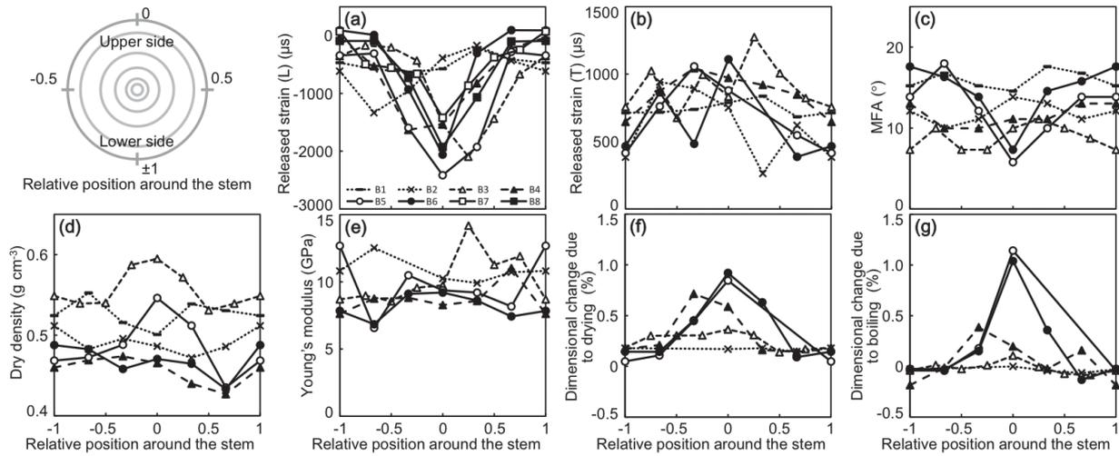
**Figure 6** Peripheral distribution of (a) released strain of growth stress in L direction, (b) released strain of growth stress in T direction, (c) MFA, (d) dry density, (e) tensile Young’s modulus, (f) dimensional changes due to drying, (g) dimensional changes due to boiling; X axis shows the relative positions around the stem, 0 = lowermost side, 1/-1 = uppermost side
