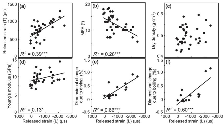
**Figure 7** Relationship between released strain of growth stress in L direction and (a) released strain of growth stress in T direction, (b) MFA, (c) dry density, (d) tensile Young’s modulus, (e) dimensional change due to drying, (f) dimensional change due to boiling; r = correlation coefficient, \* and \*\*\* = significant levels of 5 and 0.1% respectively
