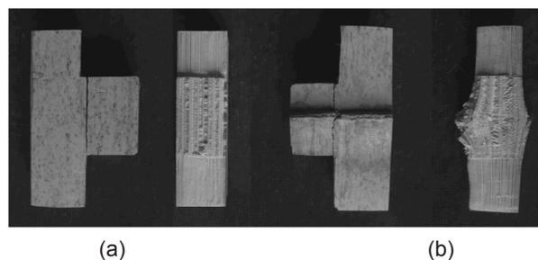
**Figure 5** Shear failure for culm (a) without node and (b) with node
