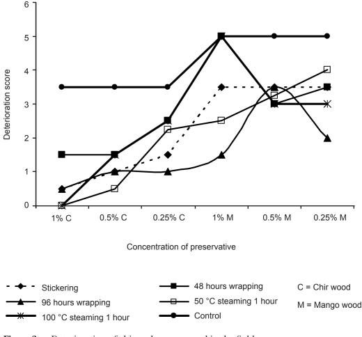
Figure 2 Deterioration of chir and mango wood in the field
