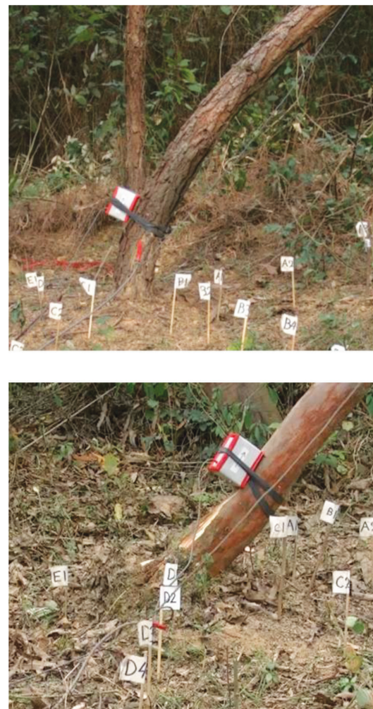
Figure 4 The flexible stem of Pinus caribaea (upper image) and tap-root broken of Eucalyptus urophylla (lower image) in the pulling experiment
