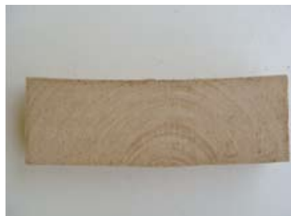
Figure 5 Cupping of an unevenly-shrunk sawn rubberwood
