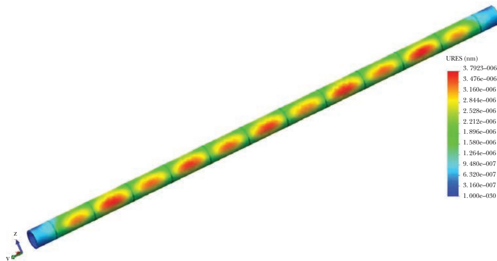
Figure 9 Bamboo culm deformation
