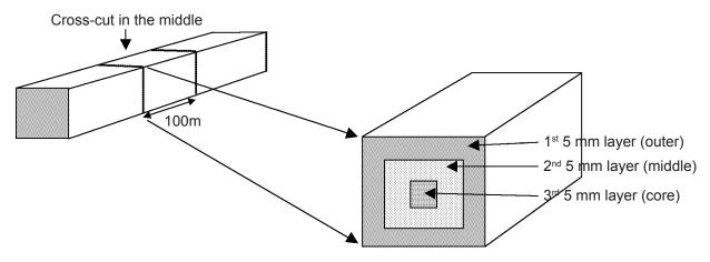
Figure 1 Sampling procedure for chemical analysis for 25 mm thick sample
