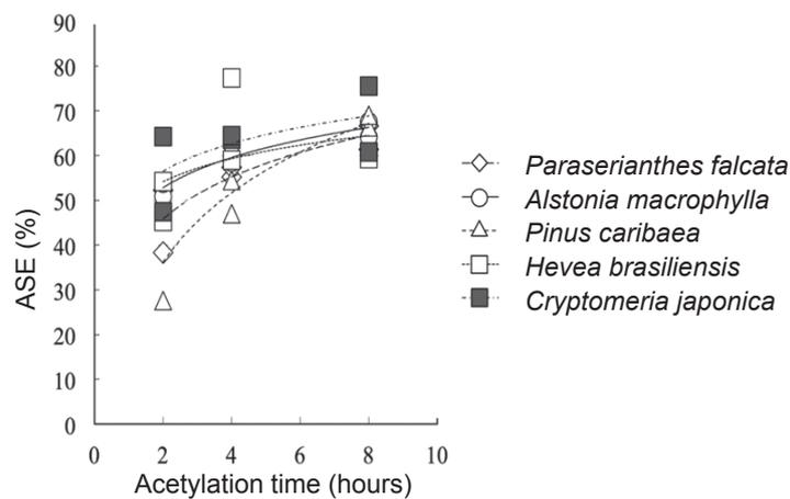
**Figure 4** Relationship between anti-swelling efficiency (ASE) and acetylation time
