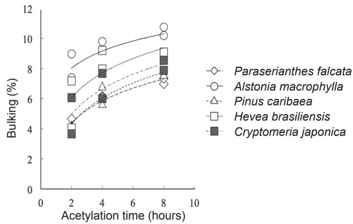
**Figure 3** Relationship between bulking and acetylation time
