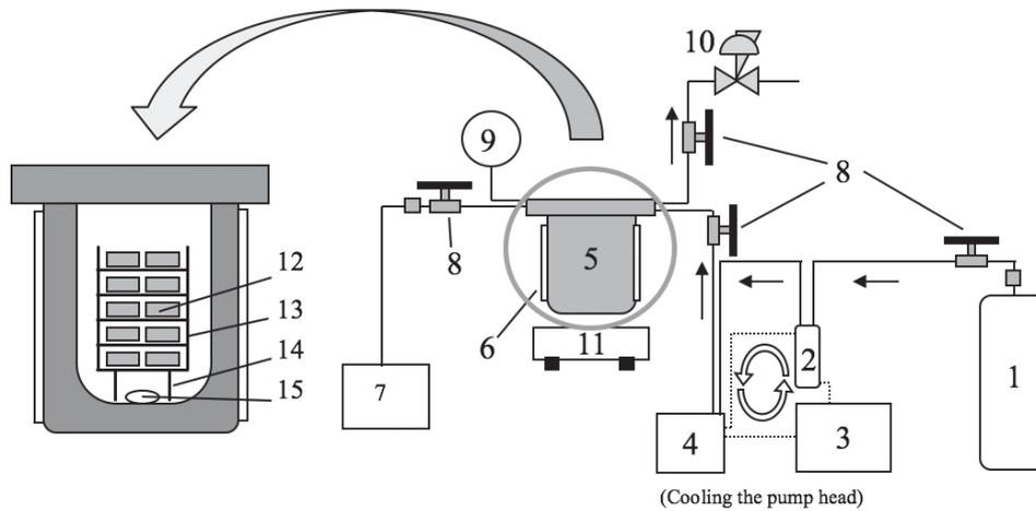
**Figure 1** Schematic diagram of supercritical CO<sub>2</sub> treatment apparatus consisting of 1: CO<sub>2</sub> cylinder, 2: condenser, 3: cold water circulator, 4: pump, 5: batch container, 6: electric heater, 7: aspirator, 8: valve, 9: pressure gauge, 10: back pressure regulator, 11: magnetic stirrer, 12: wood specimens, 13: basket, 14: acetic anhydride and 15: stirrer bar
