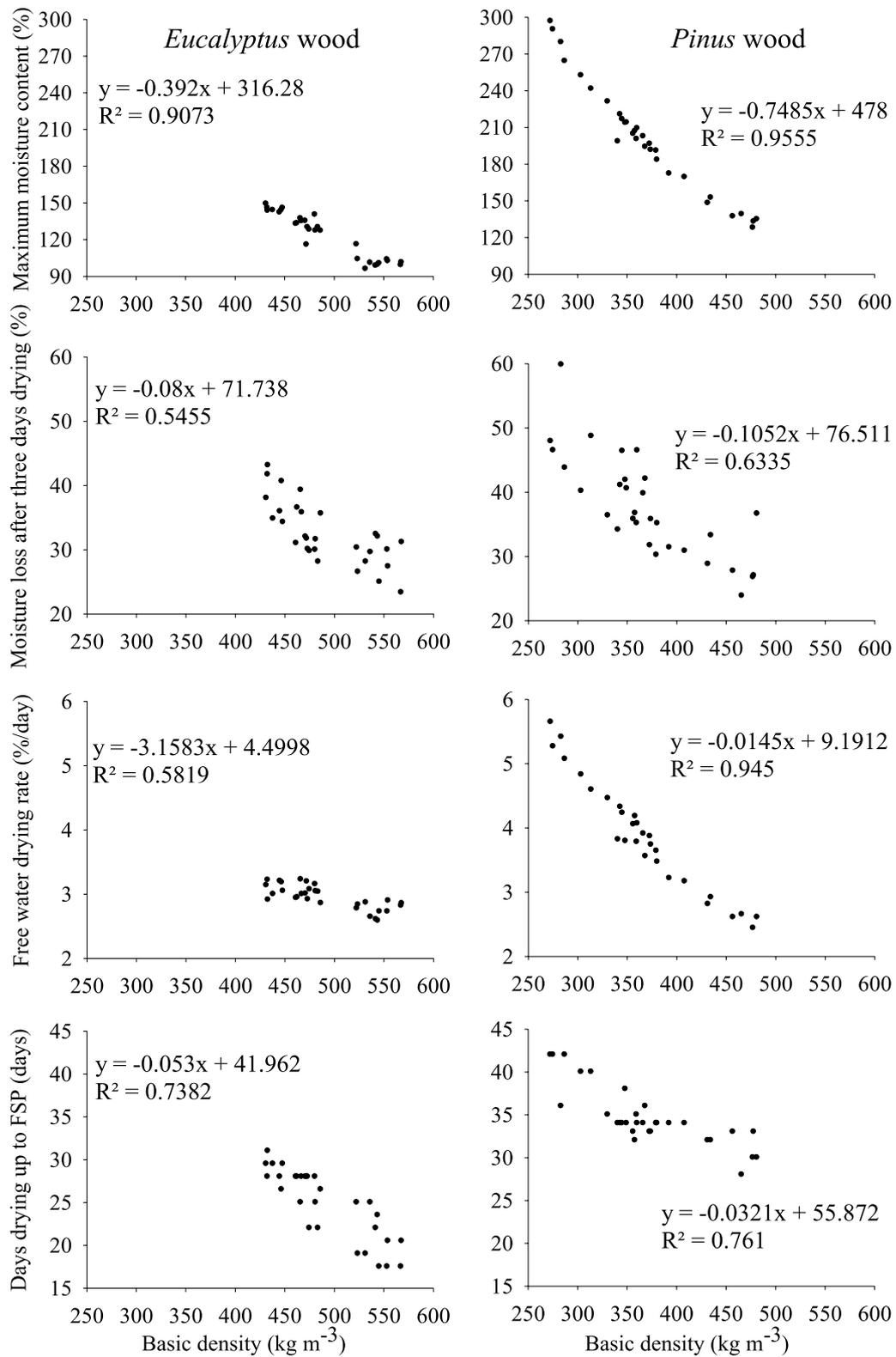
**Figure 3** Relationship between density and drying of *Eucalyptus urophylla* and *Pinus caribaea* wood above the fibre saturation point;  $R^2$  = coefficient of determination of linear regression models, SPF = fibre saturation point
