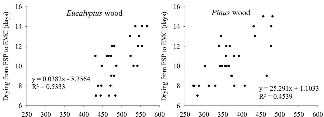
**Figure 4** Drying days between the fibre saturation point and equilibrium moisture content of *Eucalyptus urophylla* and *Pinus caribaea* wood;  $R^2$  = coefficient of determination of linear regression model, FSP = fibre saturation point, EMC = equilibrium moisture content
