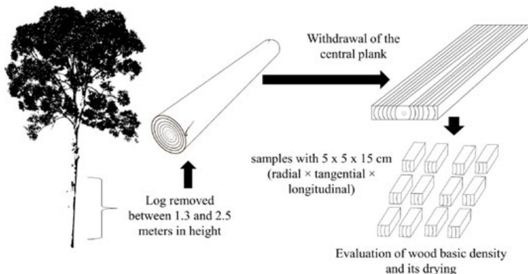
**Figure 1** Simplified diagram of sampling to evaluate wood density and its drying
