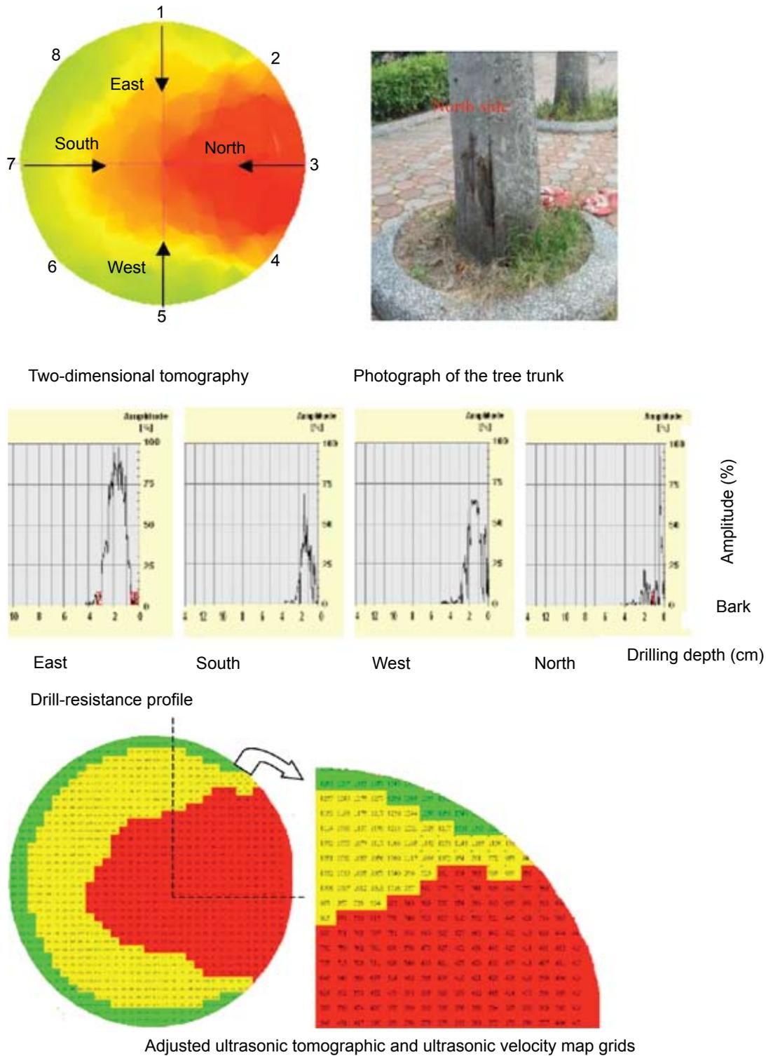
**Figure 4** Comparison of ultrasonic wave tomography and resistance profiles to verify the tomogram and a photograph of the corresponding cross-section for royal palm tree no. 16. East, south, west and north show the drilling path orientations.
