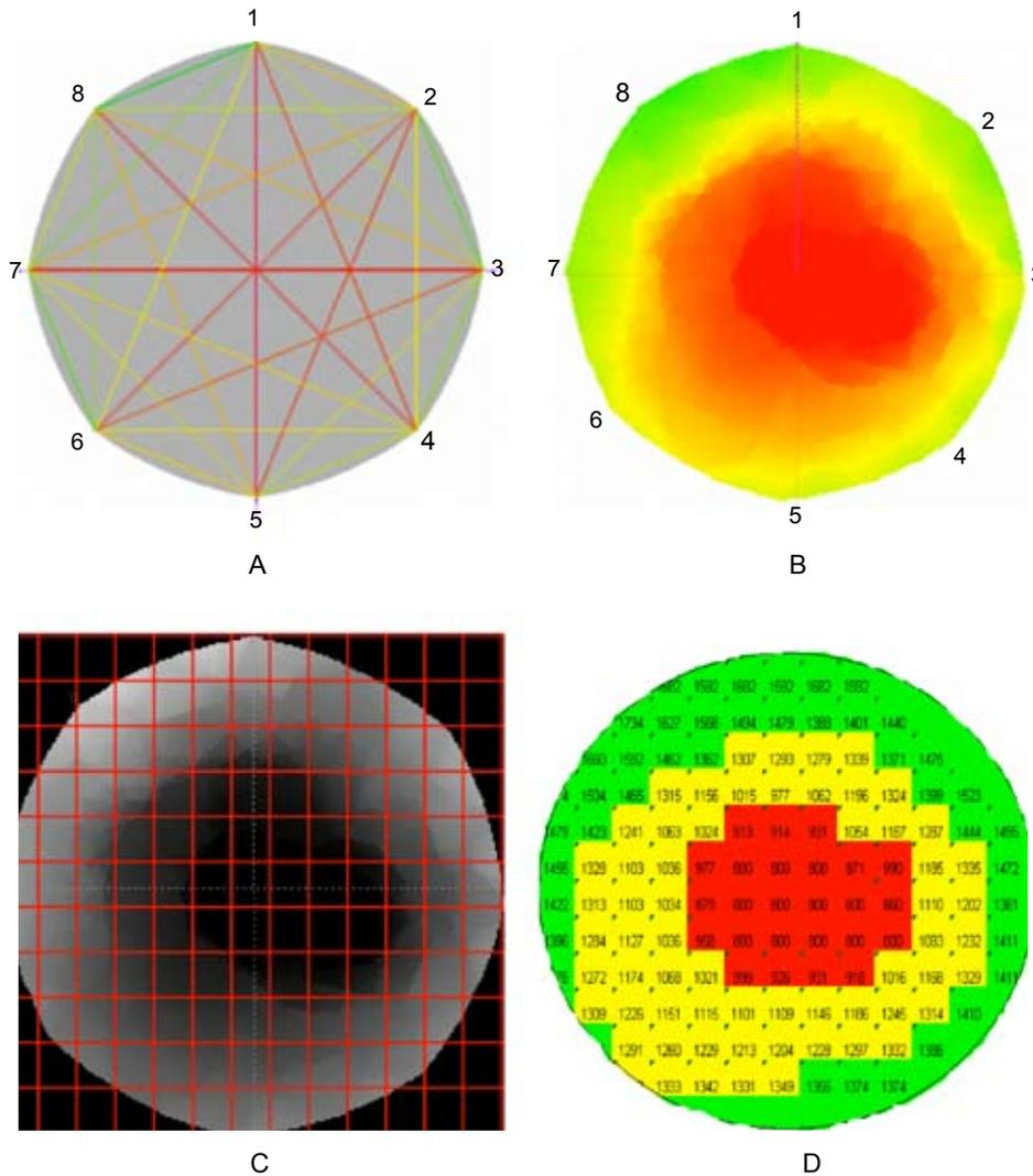
**Figure 1** Sensor arrangement, paths of ultrasonic wave measurement and 2D tomogram of the experimental procedure. Transfer procedure (from A to D) of defect evaluation: (A) acoustic tomographic test on royal palm (*Roystonea regia*) using multichannel Sylvestest ultrasonic waves (eight probes), (B) constructed 2D image by Arbotom® software, (C) conversion of the 2D image into 256 gray shades, and (D) corresponding ultrasonic wave velocity calculated for every grid square.
