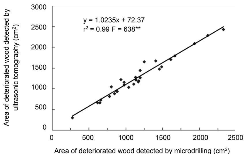
**Figure 5** Relationship between areas of deteriorated wood detected by ultrasonic tomography and microdrilling
