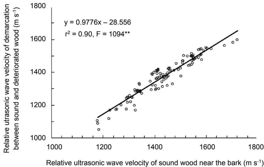
**Figure 3** Established ultrasonic wave velocity of the sound–deteriorated wood transition zone
