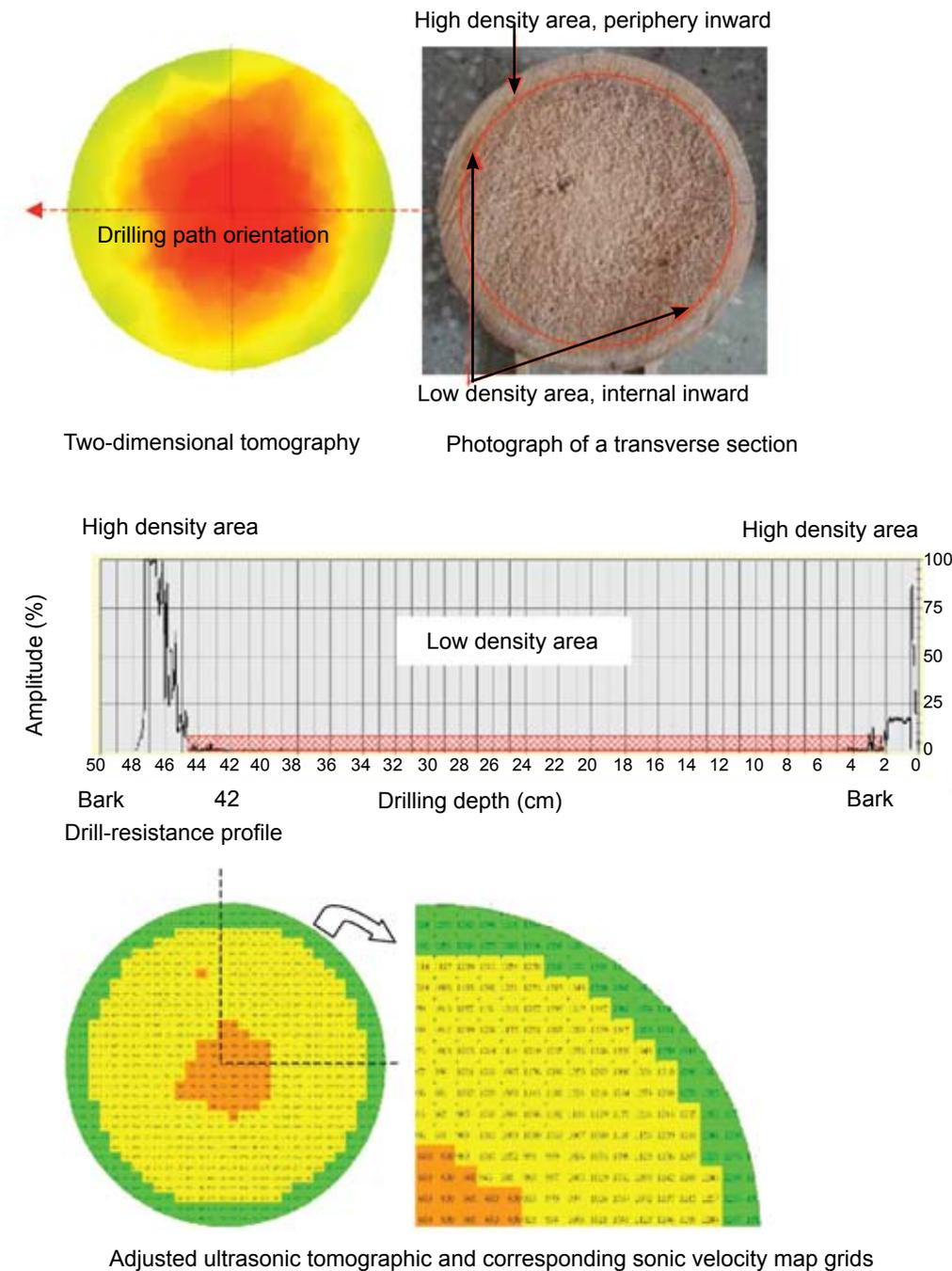
**Figure 2** Comparison of ultrasonic wave tomography and resistance profiles to verify the tomogram, and a photograph of a corresponding cross-section of royal palm disc no. 4
