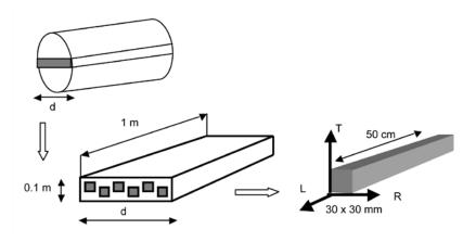
Figure 2 Localisation and size of diametrical planks and squares used
