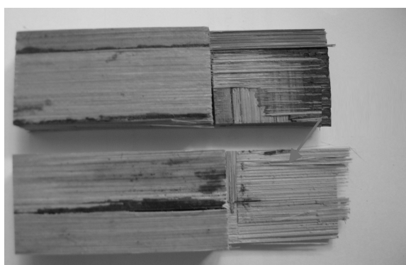
Figure 5 Bamboo failure of LMwPF-treated plybamboo
