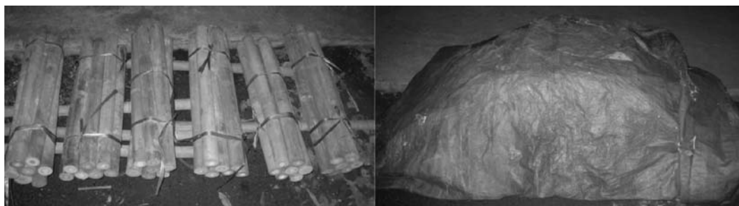
Figure 1 Bundled specimens on supports over wet soil ground and covered for infection
