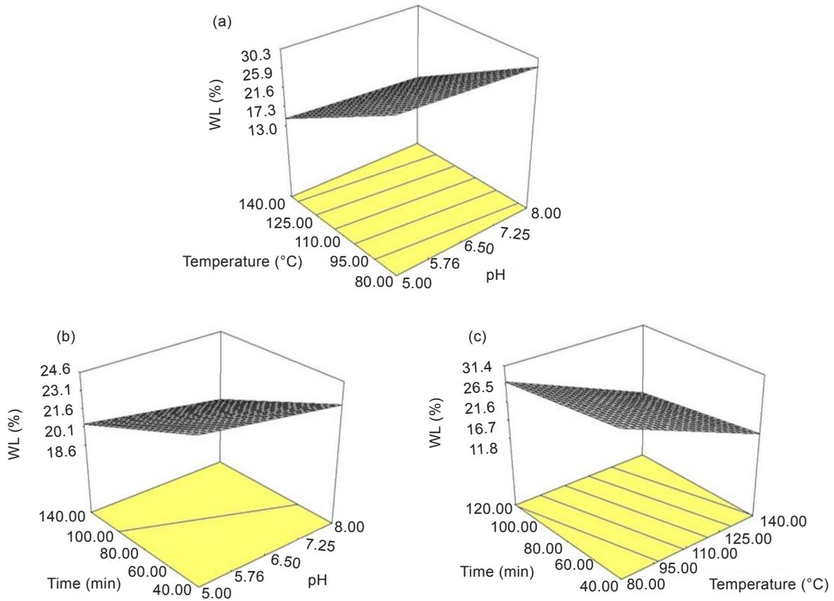
**Figure 2** 3D-surface plot of weight loss (WL) in percentage as a function of temperature and buffered pH, time and buffered pH and temperature and time
