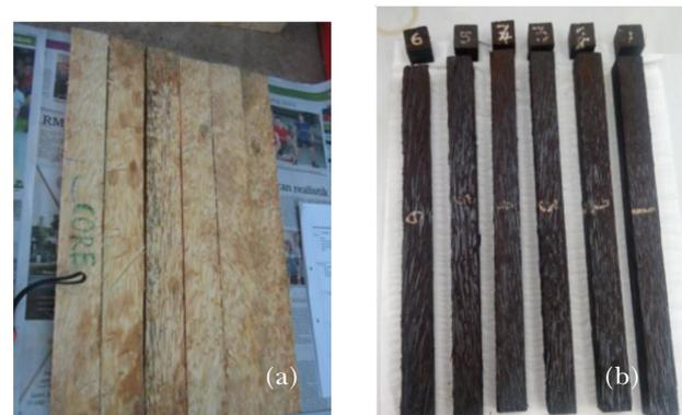
**Figure 1** Colour change in oil palm wood before (a) and after (b) hydrothermal treatment
