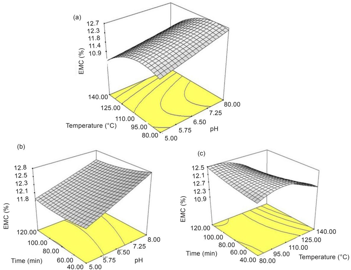
**Figure 3** 3D-surface plot of equilibrium moisture content (EMC) in percentage as a function of temperature and buffered pH, time and buffered pH and temperature and time
