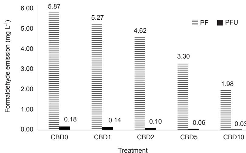
Figure 4 Formaldehyde emission of *compreg*-laminated wood after 0, 1, 2, 5 and 10 cycles of cyclic boil-dry (CBD) treatment
