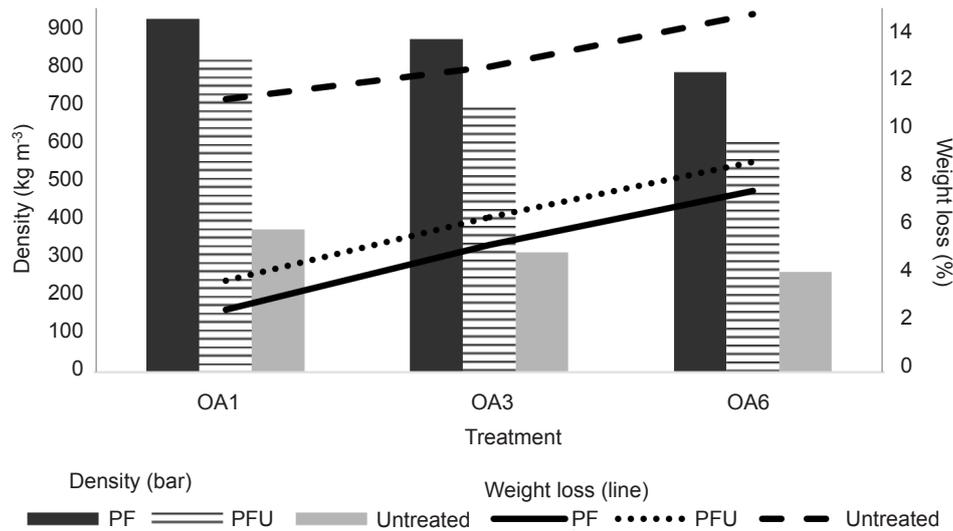
**Figure 1** Weight and density changes of *compreg* laminates after outdoor ageing (OA) for 1, 3 and 6 months
