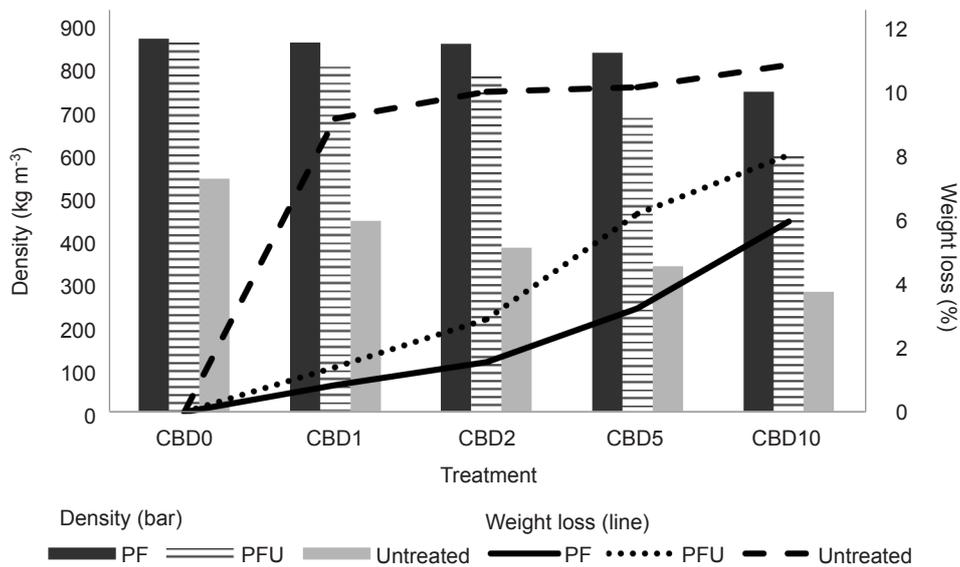
**Figure 2** Weight and density changes of *compreg* laminates after 0, 1, 2, 5 and 10 cycles of cyclic boil-dry (CBD) treatment
