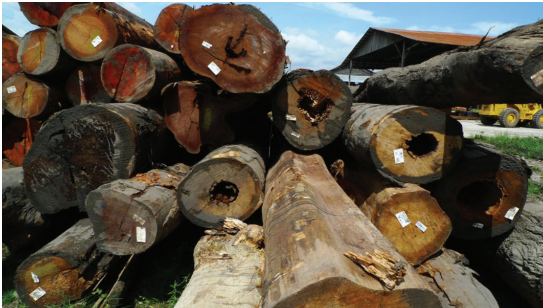
Figure 1 A stack of freshly cut logs of mixed species in a Malaysian log yard showing heartwood decay
