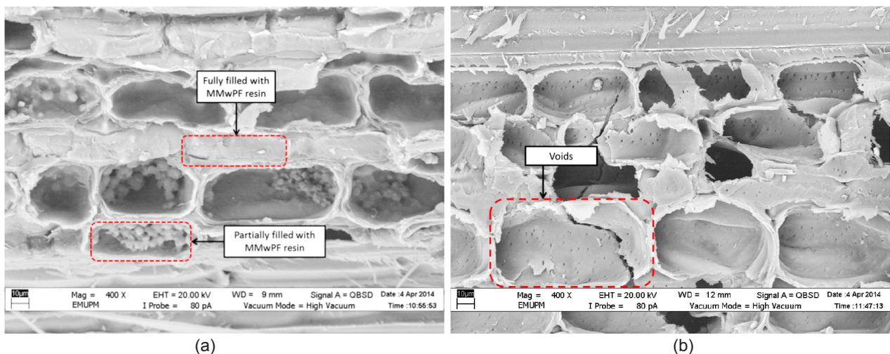
**Figure 6** Scanning electron microscope micrograph of (a) impregnated and (b) untreated bamboo sliver (400× magnification); MMwPF = medium molecular weight phenol formaldehyde
