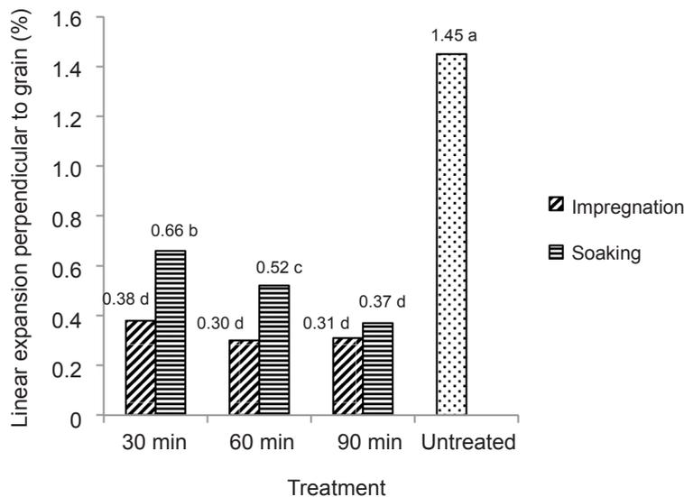
**Figure 4** Linear expansion perpendicular to grain of the samples manufactured using different treatment conditions; means followed with the same letter were not significantly different at  $p \leq 0.05$
