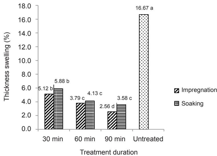
**Figure 1** Thickness swelling of the samples manufactured using different treatment conditions; means followed by the same letter are not significantly different at  $p \leq 0.05$
