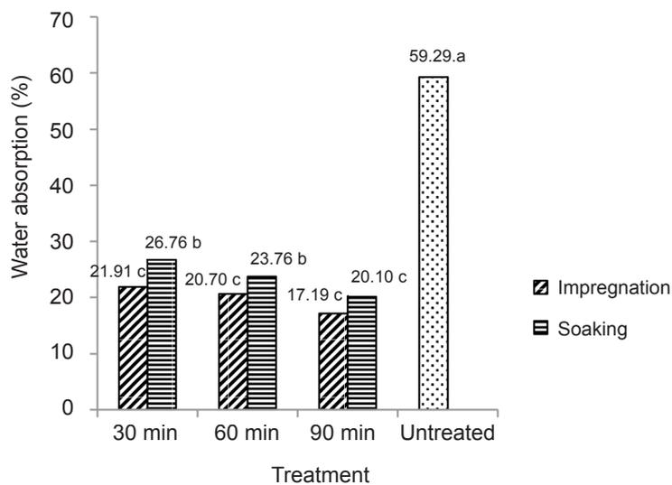
**Figure 2** Water absorption of the samples manufactured under different treatment conditions; means followed by the same letter are not significantly different at  $p \leq 0.05$
