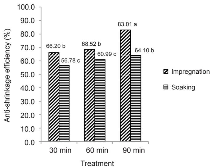
**Figure 5** Anti-shrinkage efficiency of the samples manufactured under different treatment methods and durations; means followed by the same letter are not significantly different at  $p \leq 0.05$
