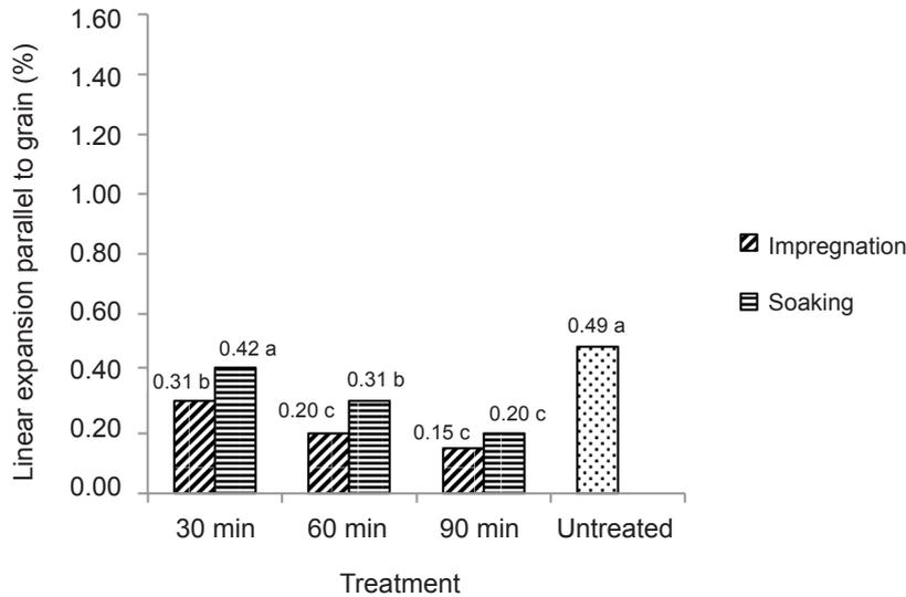
**Figure 3** Linear expansion parallel to grain of the samples manufactured using different treatment conditions; means followed by the same letter are not significantly different at  $p \leq 0.05$
