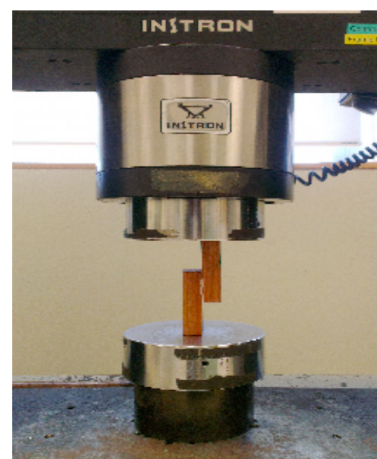
Figure 3 The set-up of the shear strength test
