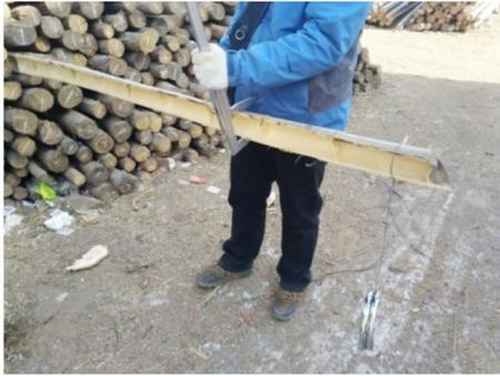
**Figure 2** Measurement of the outer diameter of the 42-node loaded bamboo
