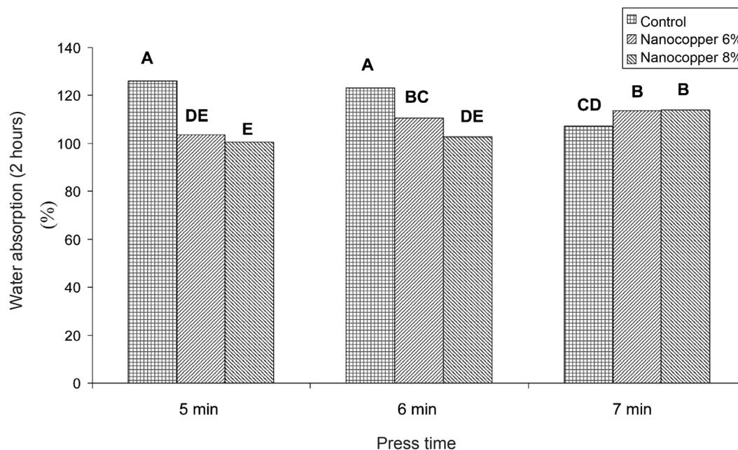
**Figure 7** Water absorption (2 hours) values at three different hot press times for each concentration of nanocopper suspension; alphabets on the columns are Duncan groupings at 99% level of confidence
