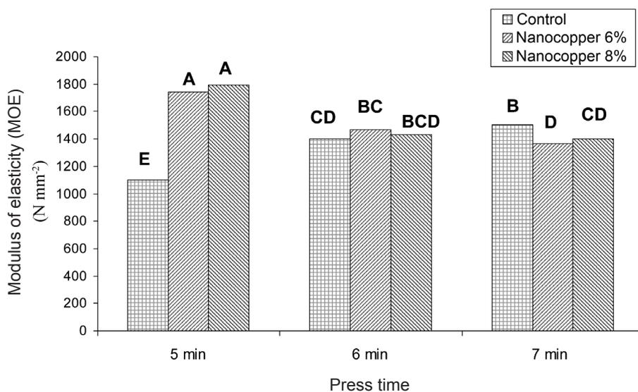
**Figure 3** Modulus of elasticity values at three different hot press times for each concentration of nanocopper suspension; alphabets on the columns are Duncan groupings at 99% level of confidence
