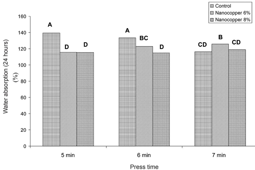
**Figure 8** Water absorption (24 hours) values at three different hot press times for each concentration of nanocopper suspension; alphabets on the columns are Duncan groupings at 99% level of confidence
