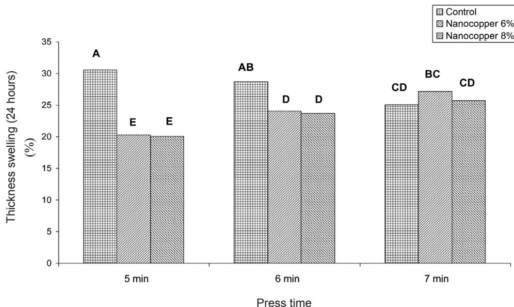
**Figure 6** Thickness swelling (24 hours) values at three different hot press times for each concentration of nanocopper suspension; alphabets on the columns are Duncan groupings at 99% level of confidence
