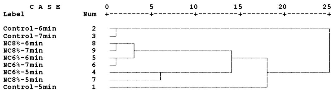
**Figure 9** Cluster analysis (Ward method) of the nine treatments, namely, three different hot press times (6, 7 and 8 min) and three concentrations of nanocopper (NC) suspension (control, 6 and 8%) based on all physical and mechanical properties (modulus of rupture, modulus of elasticity, internal bonding, thickness swelling and water absorption)
