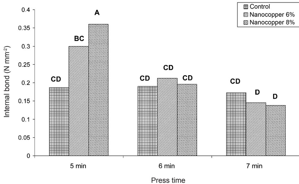
**Figure 4** Internal bonding values at three different hot press times for each concentration of nanocopper suspension; alphabets on the columns are Duncan groupings at 99% level of confidence
