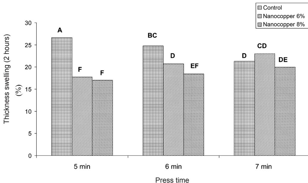
**Figure 5** Thickness swelling (2 hours) values at three different hot press times for each concentration of nanocopper suspension; alphabets on the columns are Duncan groupings at 99% level of confidence
