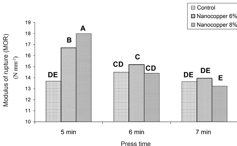
**Figure 2** Modulus of rupture values at three different hot press times for each concentration of nanocopper suspension; alphabets on the columns are Duncan groupings at 99% level of confidence
