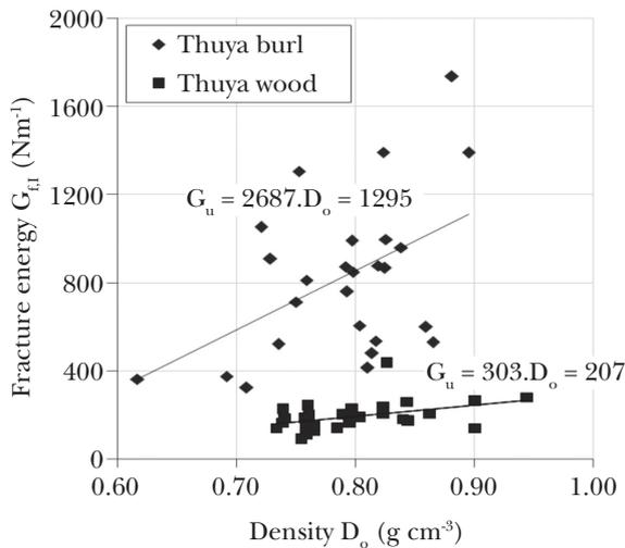
**Figure 9** Relation between fracture energy and oven-dry density
