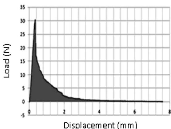
Figure 8 Force–displacement curve for thuya wood in TL system
