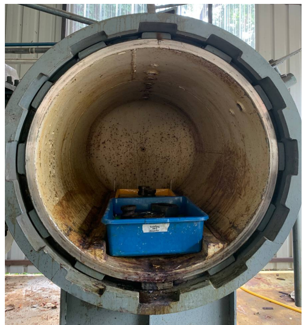
Figure 3 Impregnation modification process by using vacuum chamber
