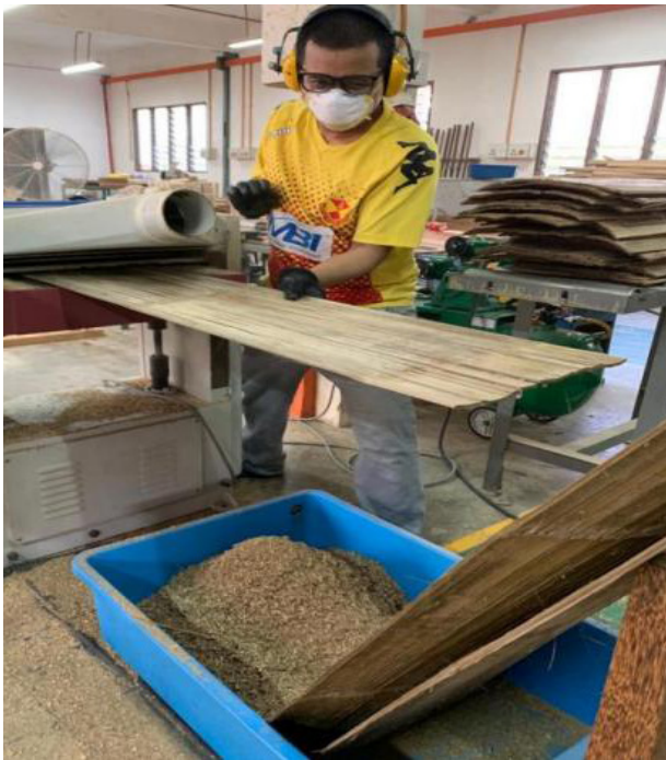
Figure 1 Planing process of bamboo veneer
