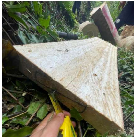
Figure 7 Occurrence of splitting after crosscutting and sawing logs into boards; a S-shaped metal plate is fixed to prevent further splitting
