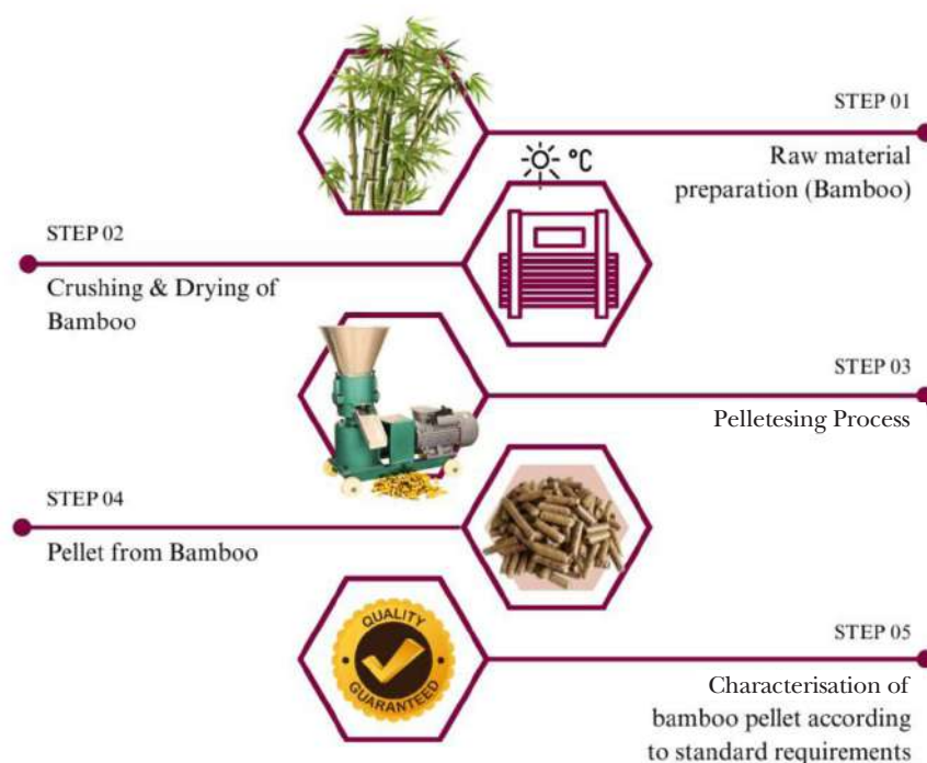
Figure 3 Production of bamboo pellets using pelletising machine
