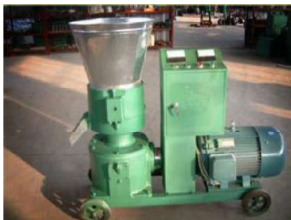
Figure 2 Laboratory-scale pelletising machine
