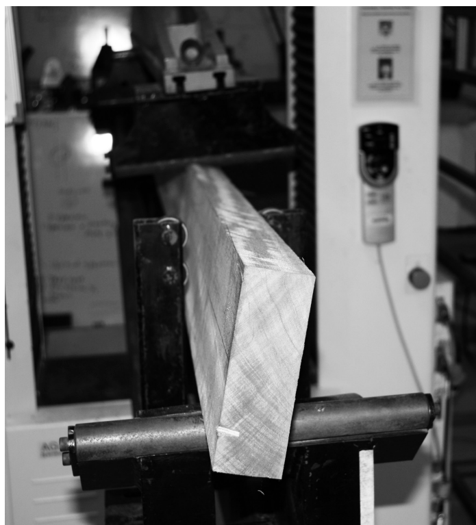
Figure 8 Twisted specimen during test
