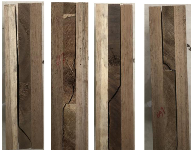
Figure 6 Failure mode of acacia CLT blocks under the planar shear test
