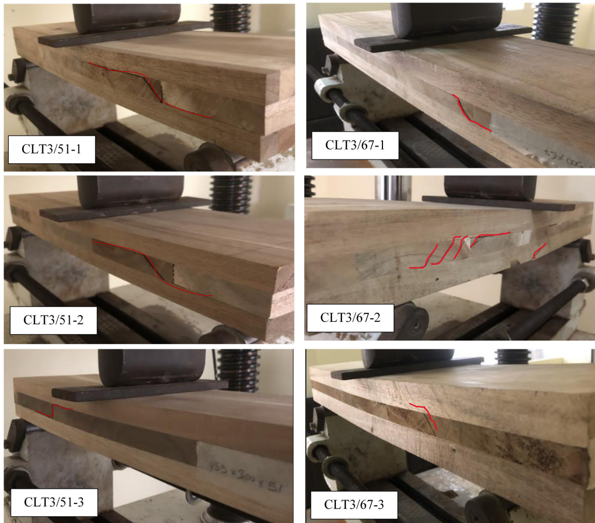
Figure 4 Failure modes of three-layer short-span acacia CLT samples under three-point bending tests
