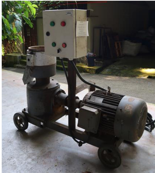
Figure 2 Pelletiser machine of a capacity of 100 kg h -1 equipped with rotating roller-cylinders
