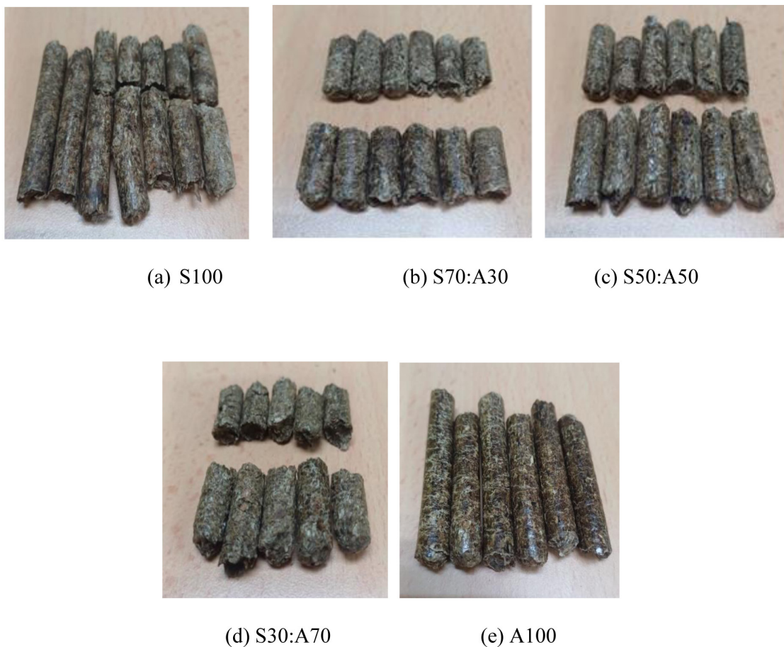
Figure 4 Sago- Acacia mangium biofuel pellet, 8 mm diameter (a) S100, (b) S70:A30, (c) S50:A50, (d) S30:A70, and (e) A100 (A = A. mangium , S = sago bark)
