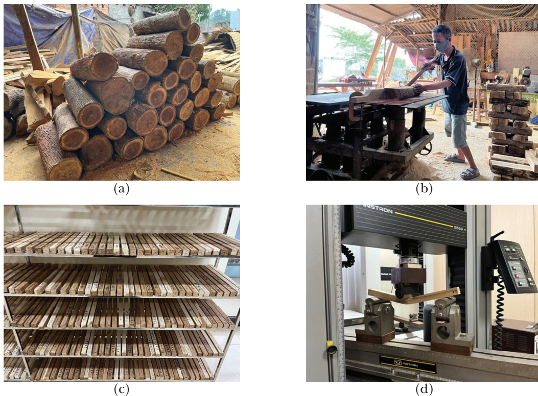
Figure 2 The experimental procedures: 50-cm-long logs from five sampled trees (a), specimen cutting (b), static bending strength specimens (c), destructive testing (d)
