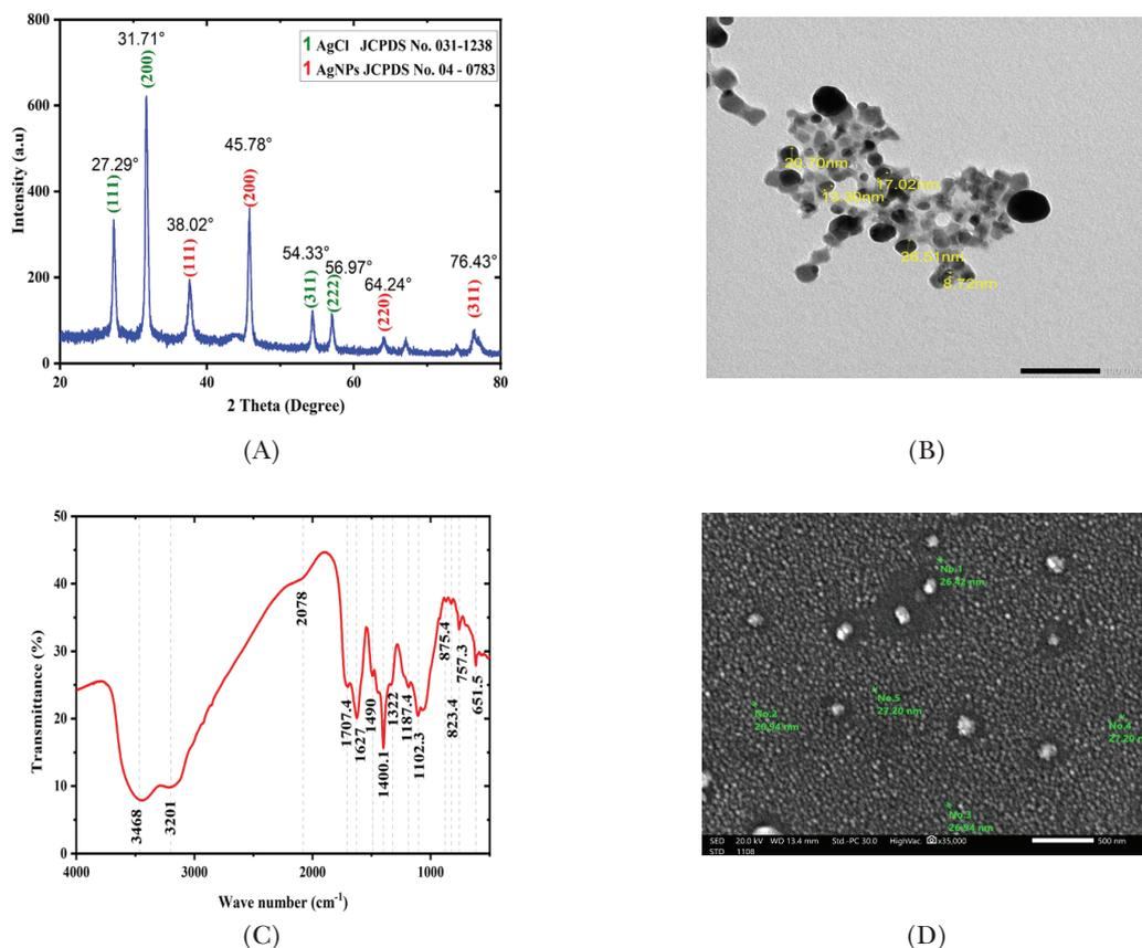
**Figure 3** Characterisation of biogenic silver nanoparticles (AgNPs). (A) X-ray pattern with peak indices and 2-theta position; (B) Transmission Electron Microscopy TEM, (C) Fourier Transform Infrared Spectroscopy FTIR and (D) Scanning Electron Microscopy SEM
