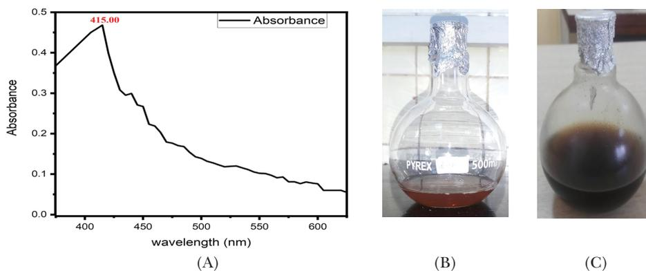
**Figure 2** UV-visible spectroscopy of biogenic silver nanoparticles (A), *Eucalyptus camaldulensis* plant extract (B), The formation of a blackish-brown color indicates the formation of silver nanoparticles (C)
