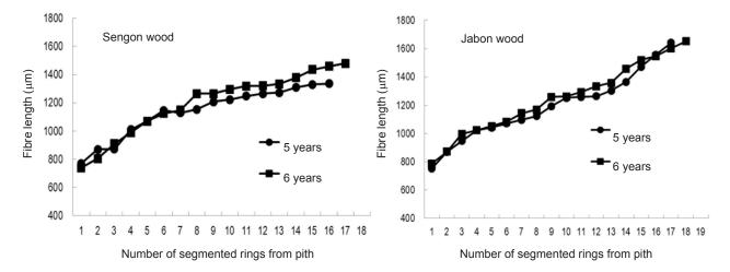
Figure 4 Comparison of radial variation of average fibre length in 5- and 6-year-old sengon and jabon
