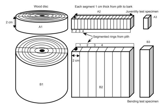
Figure 1 Schematic drawing of the preparation of the juvenility and bending test specimens (Darmawan et al. 2013)
