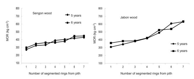
Figure 6 Comparison of radial variation of average modulus of rupture (MOR) in 5 and 6-years old sengon and jabon
