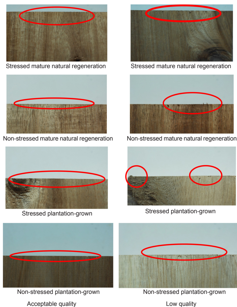
Figure 2 Surface quality of stressed and non-stressed wood after sawing test; clean surface cut signifies acceptable quality (left) while unclear surface cut signifies low quality (right)
