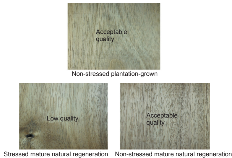
Figure 3 Surface quality of stressed and non-stressed wood after planing test
