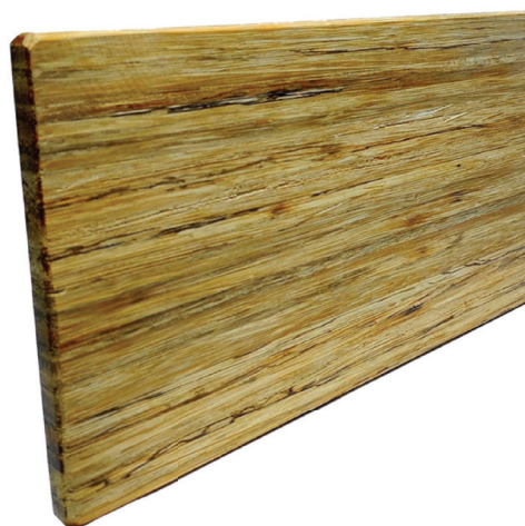
Figure 6 Prototype of a cutting board made with glued açai palm wood; source: Batista et al. (2022)
