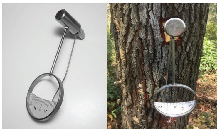
**Figure 2** Measurement device for measuring grain angle of standing trees; On the measurement scale “H” and “V” indicate right-handed and left-handed spiral grain, respectively
