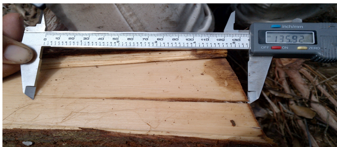
Figure 9 Split length measurement for splits from pith to bark of \geq 1 mm width (135.92 mm)
