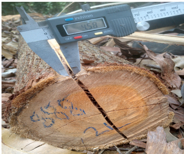
Figure 5 Measurement of split width (4.58 mm) for splits from pith to bark \geq 1 mm width
