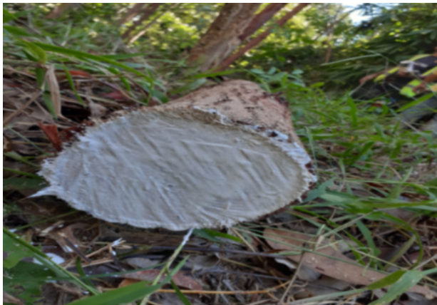
Figure 11 Application of wax emulsion (Anchorseal 2) at log end
