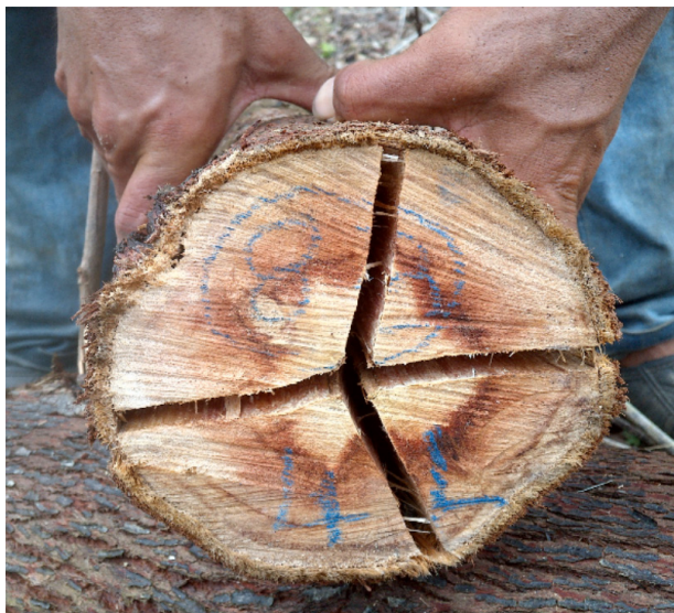
Figure 7 Severe splitting of family 88
