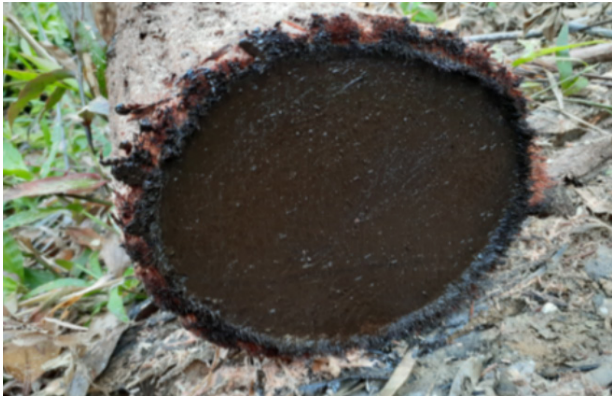
Figure 12 Application of bitumen paste (Atlaskote 103) at log end
