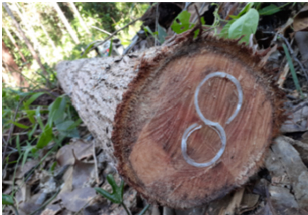
Figure 10 Plastic s-hook applied to the cut surface
