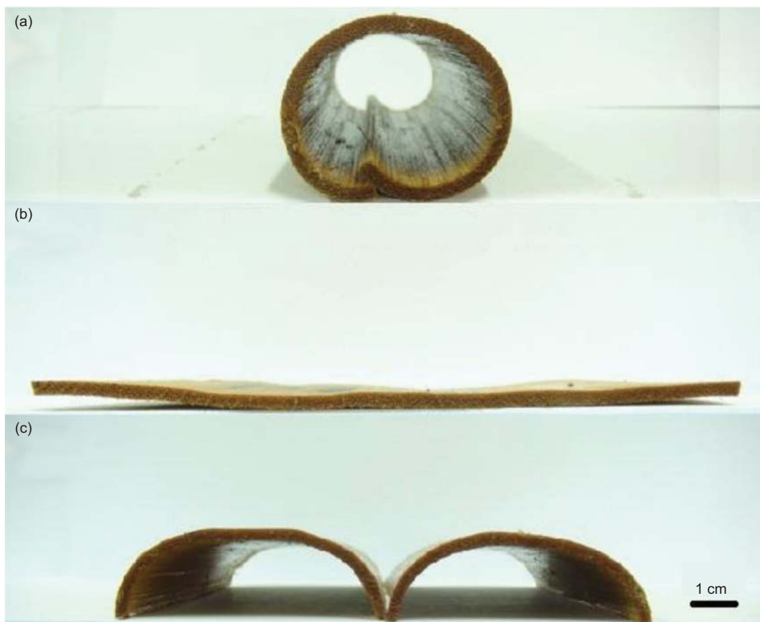
Figure 3 Photographs showing (a) rolled, (b) flat and (c) broken specimens of half tubular bamboo specimens obtained after the flattening process in hot linseed oil
