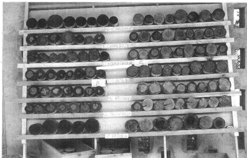
Figure 1. Cross-sections of poles treated by sap-replacement (right) and pressure impregnation (left). Near the middle of each row (species) is the best treated specimen of either method, followed immediately by the worst and so on paired
