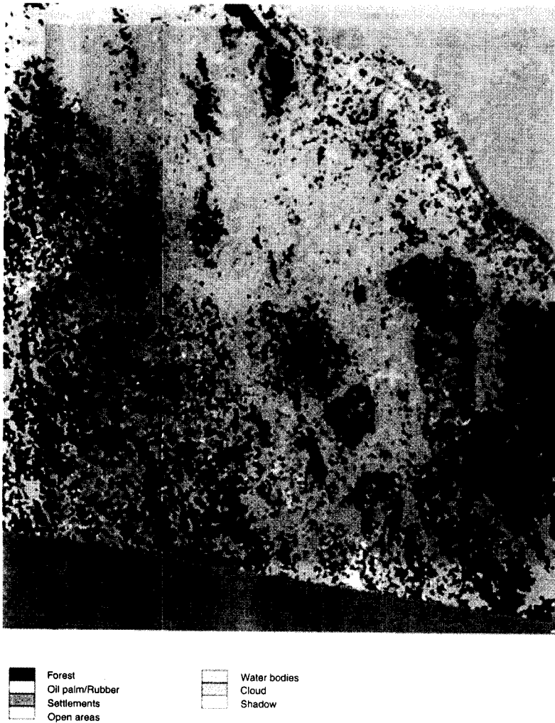
Figure 3 Unsupervised image classification for deforested area of northern Kelantan with mode filtering using isodata classifier
