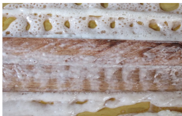
Figure 2 Glue burrs on a side face of a mixed difou-abura glulam beam
