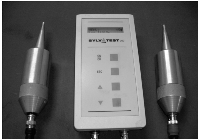
Figure 3 Non-destructive ultrasonic device SylvatestDuo
