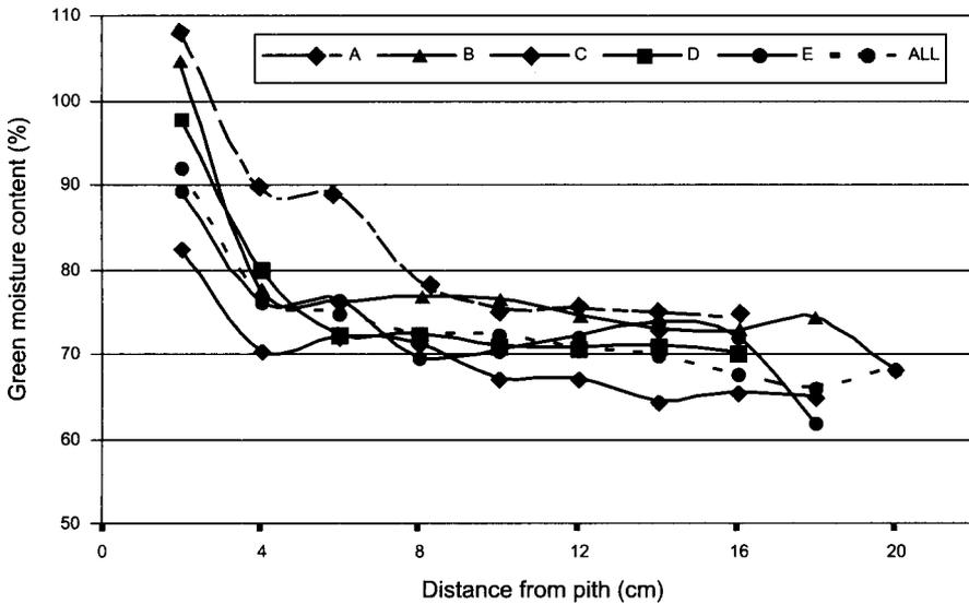
Figure 1 Radial green moisture content profile of cedrela from Ghana
