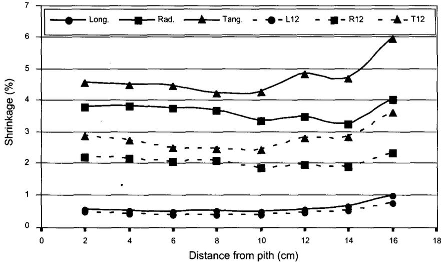
Figure 3 Shrinkage profile from pith to bark of cedrela from Ghana
