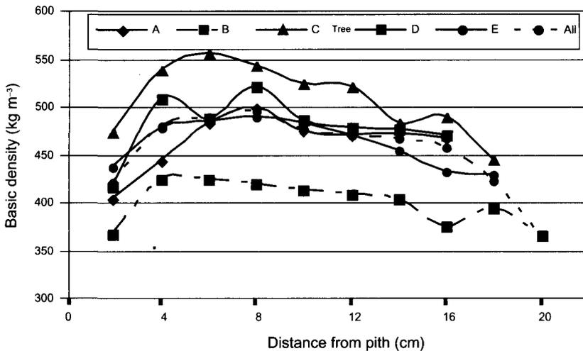
**Figure 2** Radial variation in basic density of cedrela from Ghana
