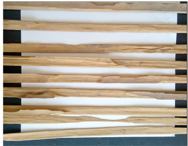
Figure 2 Bamboo test samples showing damage from Subterranean termite attack
