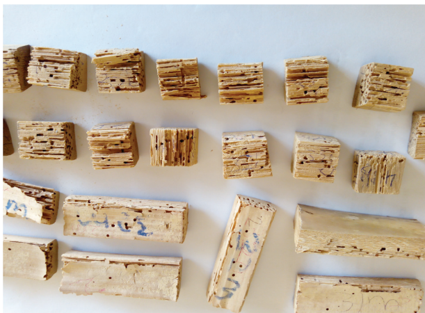
Figure 1 Bamboo test blocks showing damage from powder-post beetle attack
